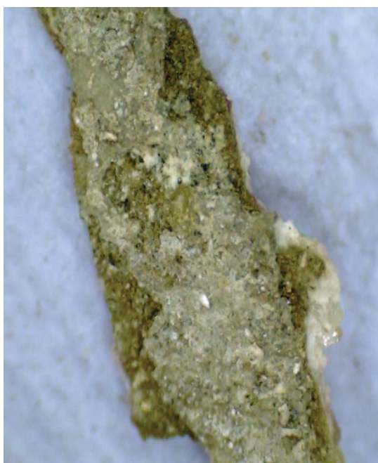
Figure 11. Sample 5. An overhead projection shows the deposition layer of discoloured lime wash and added pollutants. (x 200 magnification)
