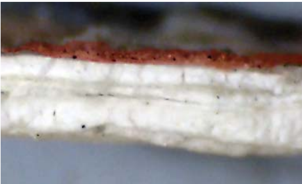
Figure 9. Sample 4. At x 200 magnification the multiple paint layers can be noted. The underlying plain limewash layers suggest that the red pigment is not original to the building, but forms part of the later decoration to this entry area.
