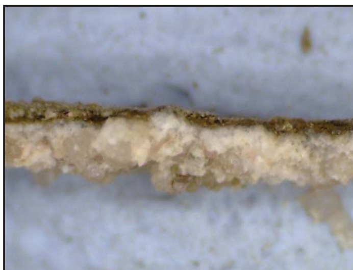
Figure 12. Sample 5. This rather concentrated green pigment is likely to be a green earth, a common material in use from the 12th to 19th centuries. (x 200 magnification)
