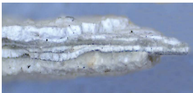
Figure 5. Sample 2. In cross-section showing at least 6 limewash layers, interleaved with soot particles; and the stone support. (x 200 magnification).
