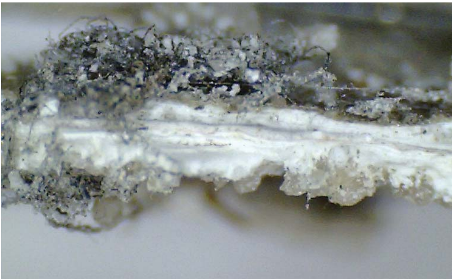
Figure 2. Sample 1. Stratigraphy in cross-section at x 200 magnification shows surface accumulations of microbiological fungal hyphae; soot and dust particles; salt crystals; and up to 6 limewash layers; and stone support.
