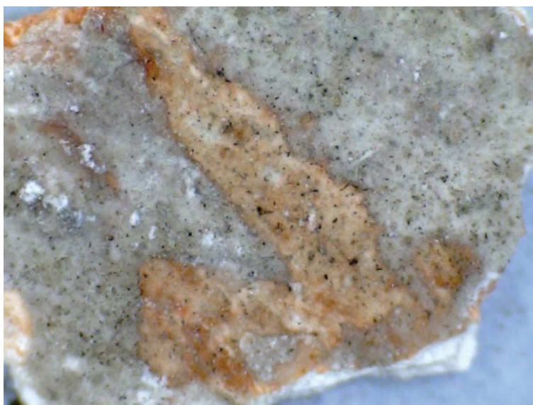
Figure 7. Sample 3. At x 200 magnification this surface aspect reveals soot particles; overlying limewash layer; a red paint layer; and ground.
