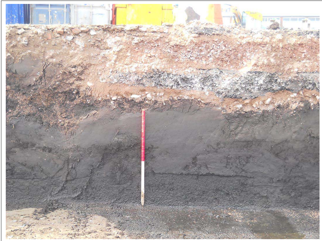
Plate 10: View of sample section within Area 3 showing disturbed rubble overburden above deeper peat deposit. Scale 1x1m
