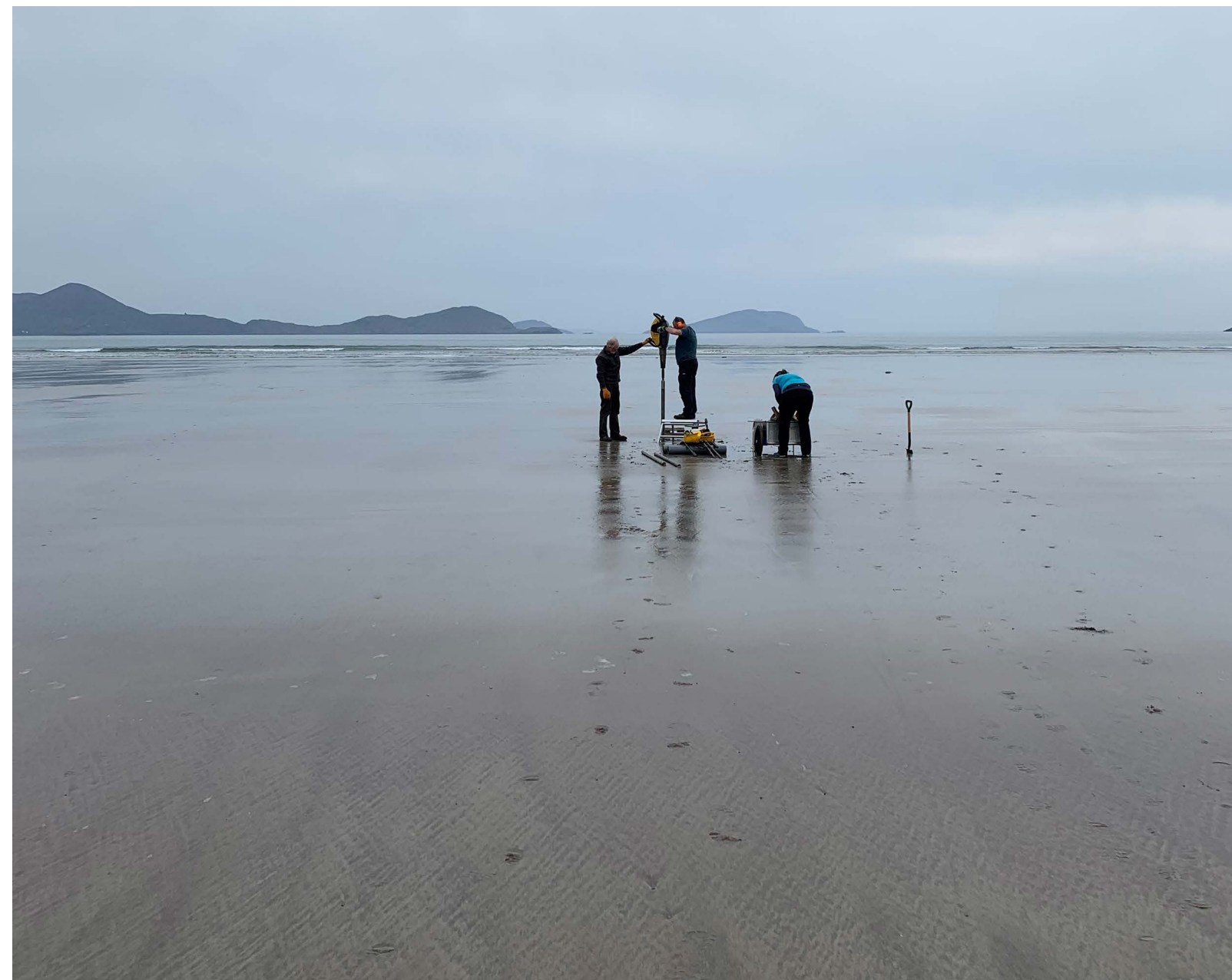
Percussion coring of the submerged landscape at Ballinskelligs. Croileacú cnagtha de thirdhreach báite ag Baile an Sceilig.
