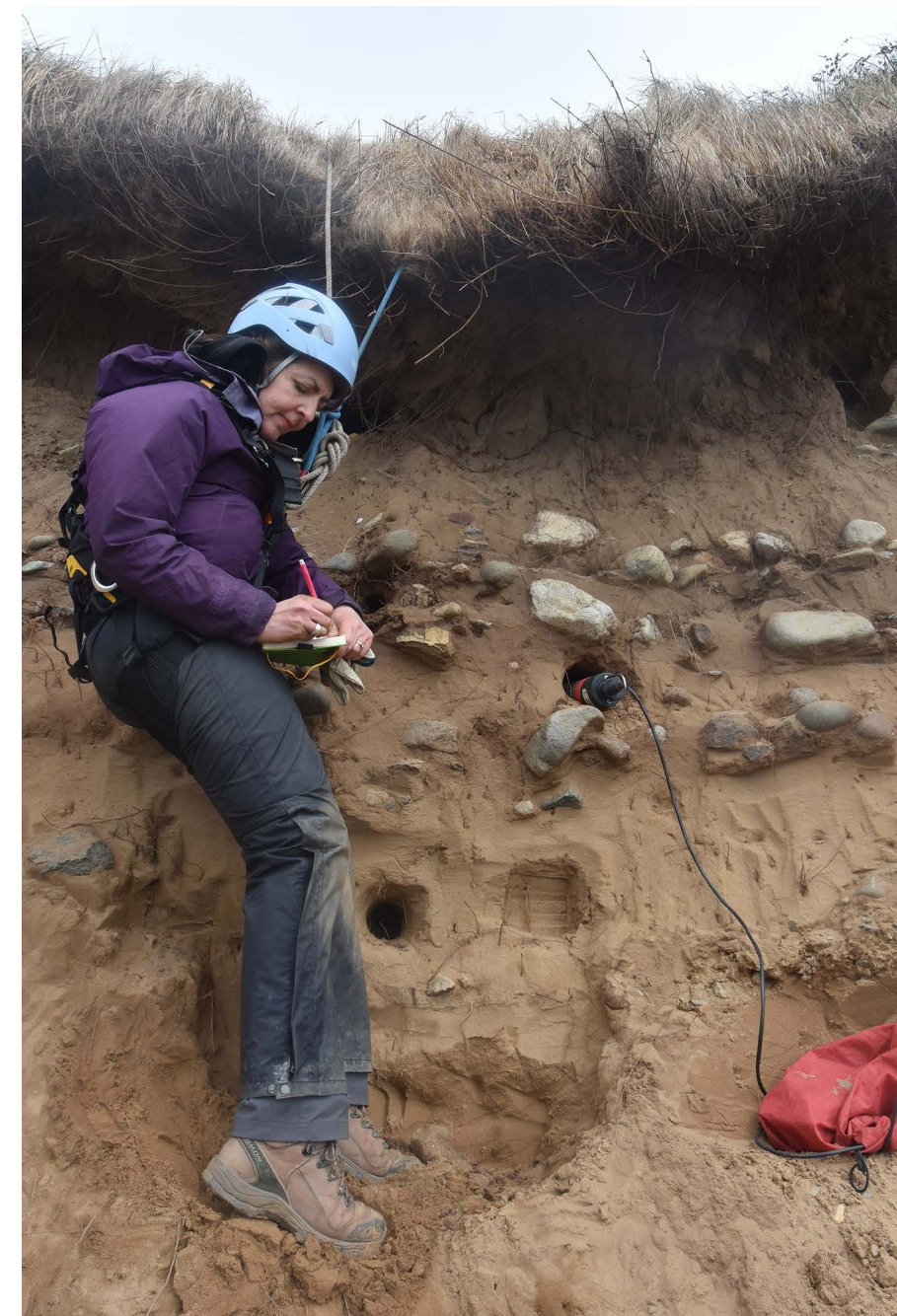
Helen retrieving OSL (Optical Stimulated Luminescence) samples from the cliff face at Dinas Dinlle.
