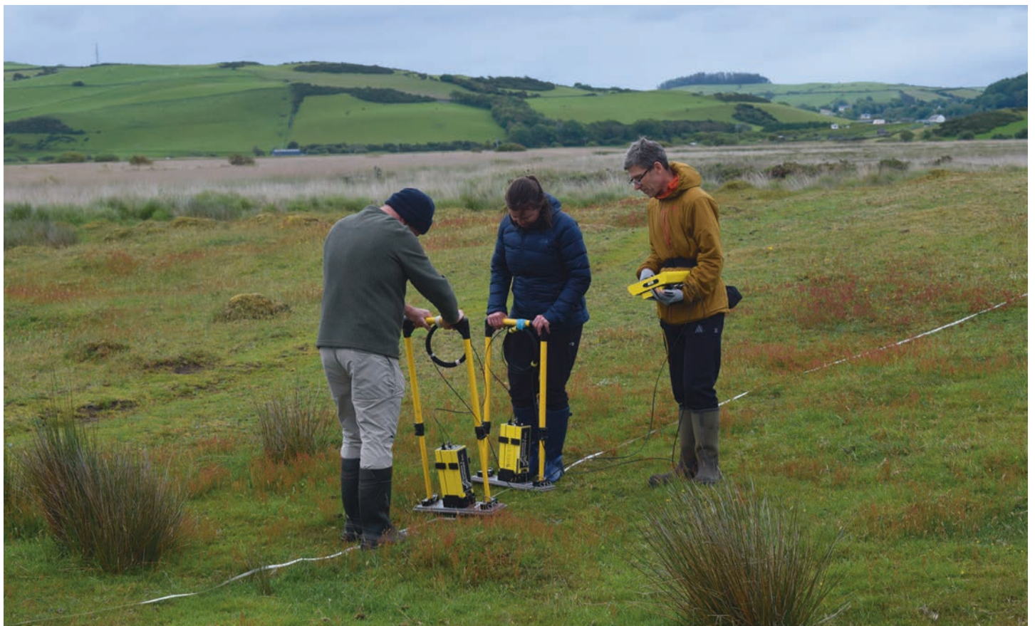
Charlie Bristow a Lucy Beck yn cymryd mesuriadau radar treiddio'r ddaear ar ymyl tafod Y Borth gyda chymorth y tîm CHERISH. Charlie Bristow and Lucy Beck conducting ground penetrating radar measurements on the edge of the Borth spit with assistance from the CHERISH team.
