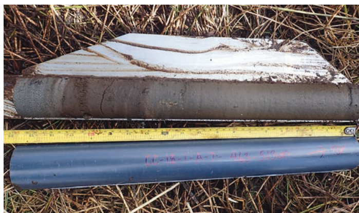
A sediment sample obtained with a Russian corer from Castlemartin Corse, Pembrokeshire. This sample is from c. 5 metres below the ground.
