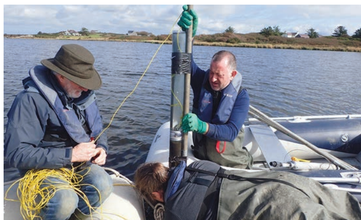
Retrieving a surface sediment core from Llyn Maelog. Croileacán dríodar dromchla á fháil ó Llyn Maelog.
