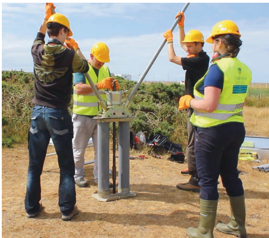
Retrieving a percussion core sample near Borth, Ceredigion. Sampla croileacán tuargana á fháil i ngar do Borth, Ceredigion.
