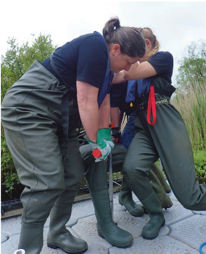
Pushing the Livingstone corer into the sediments at Stackpole Mere, Pembrokeshire.
