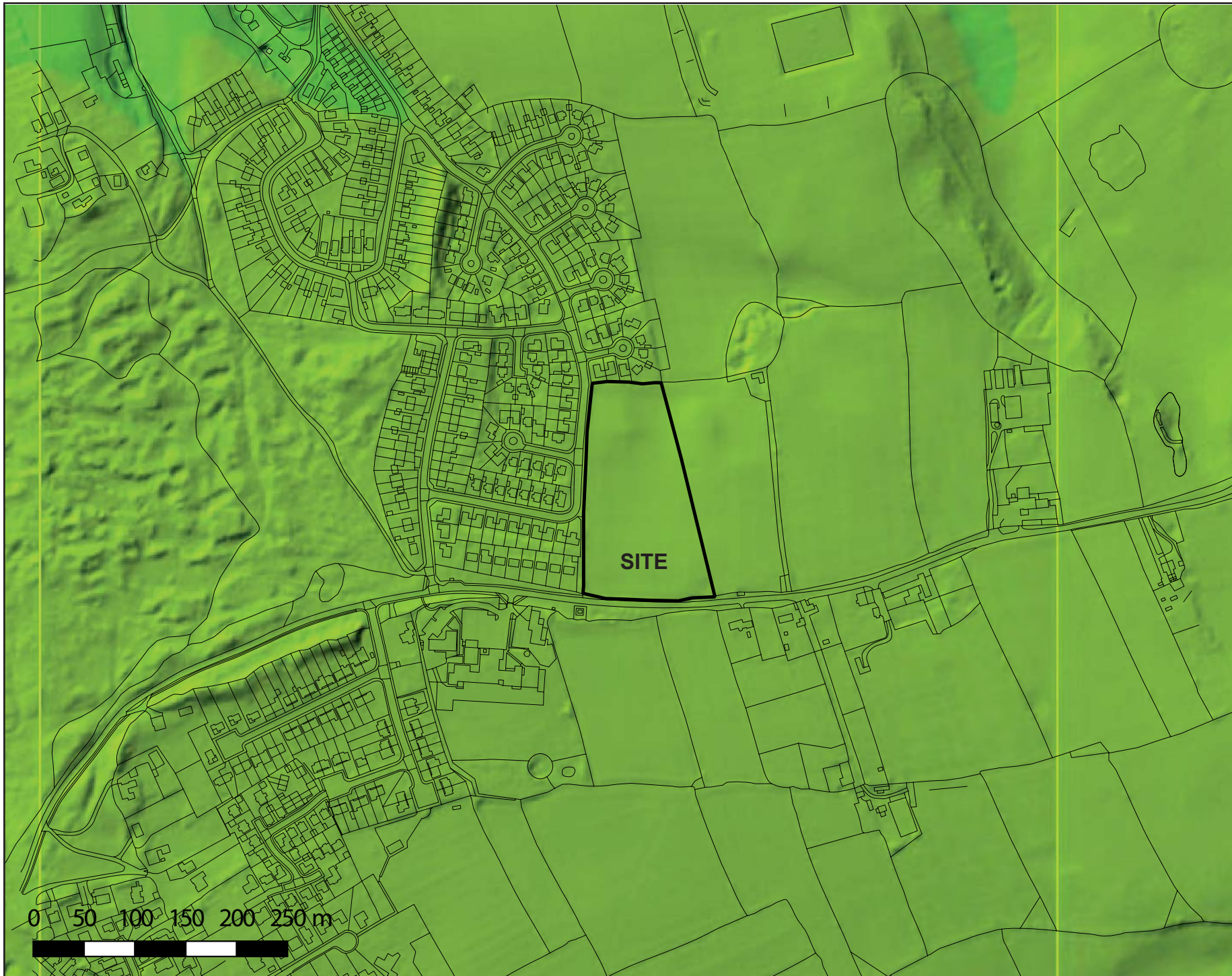
Figure 7: Lidar data at 2m DTM, overlaid with mapping detail and site location.
