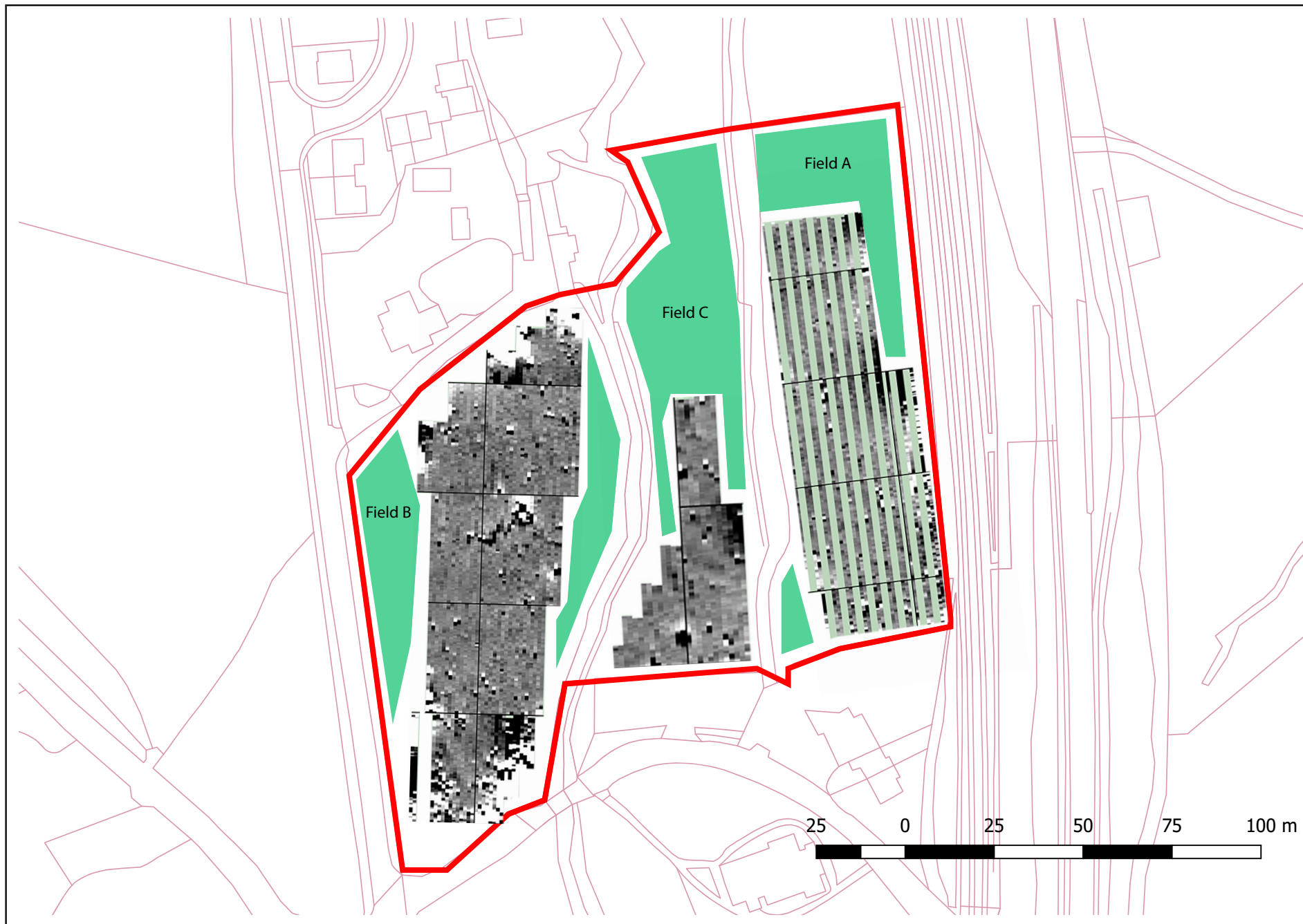
Figure 3. Showing magnetometer data clipped at -2nT to 2nT. Green shows inaccessible areas due to vegetation. Site centred on NGR SO 31146 16468.
