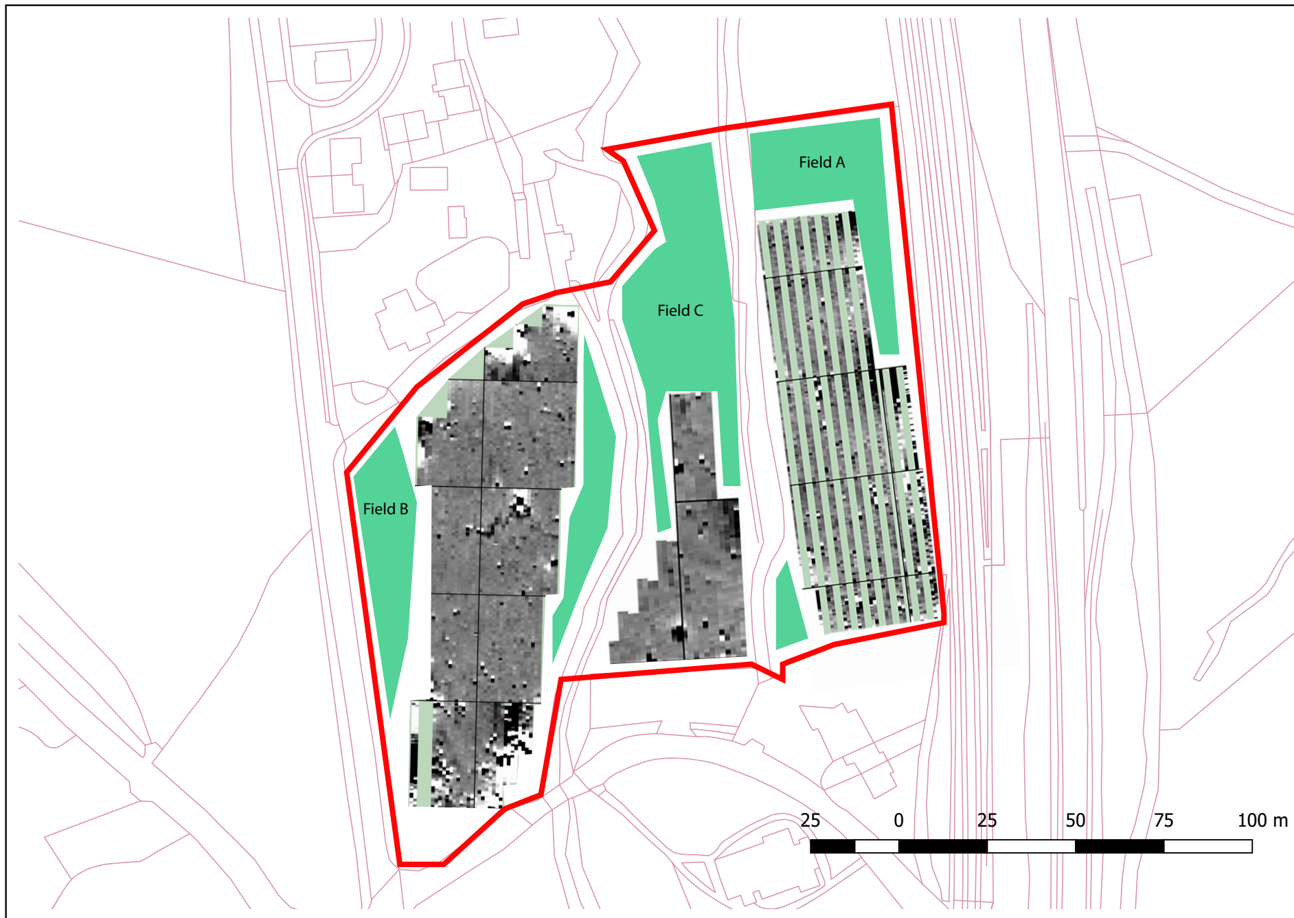
Figure 2. Showing magnetometer data clipped at -3nT to 3nT Green shows inaccessible areas due to vegetation Site centred on NGR SO 31146 16468
