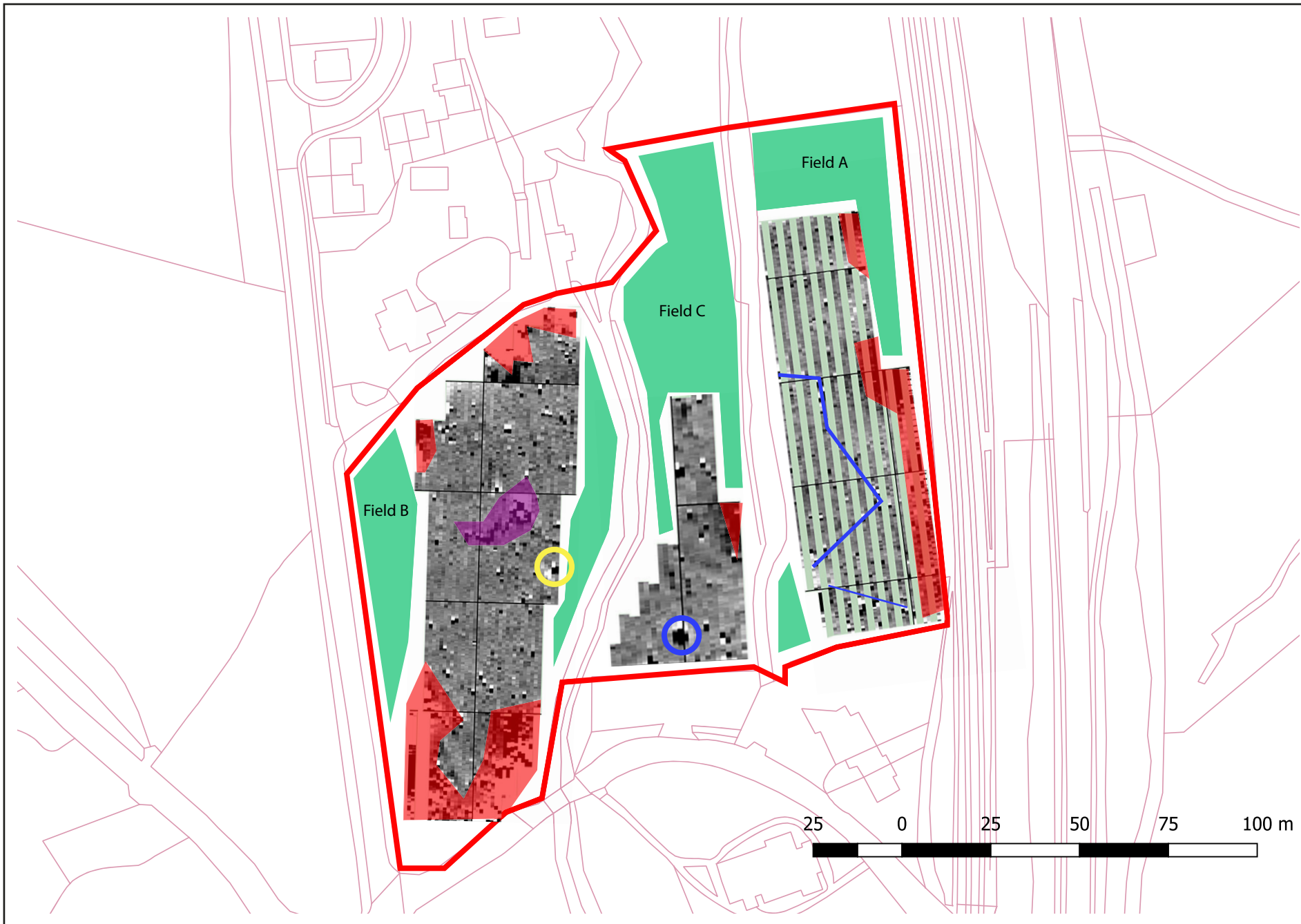
Figure 4. Showing magnetometer data clipped at -2\text{nT} to 2\text{nT} . Green shows inaccessible areas due to vegetation Site centred on NGR SO 31146 16468. Interpretation overlay described in Section 4
