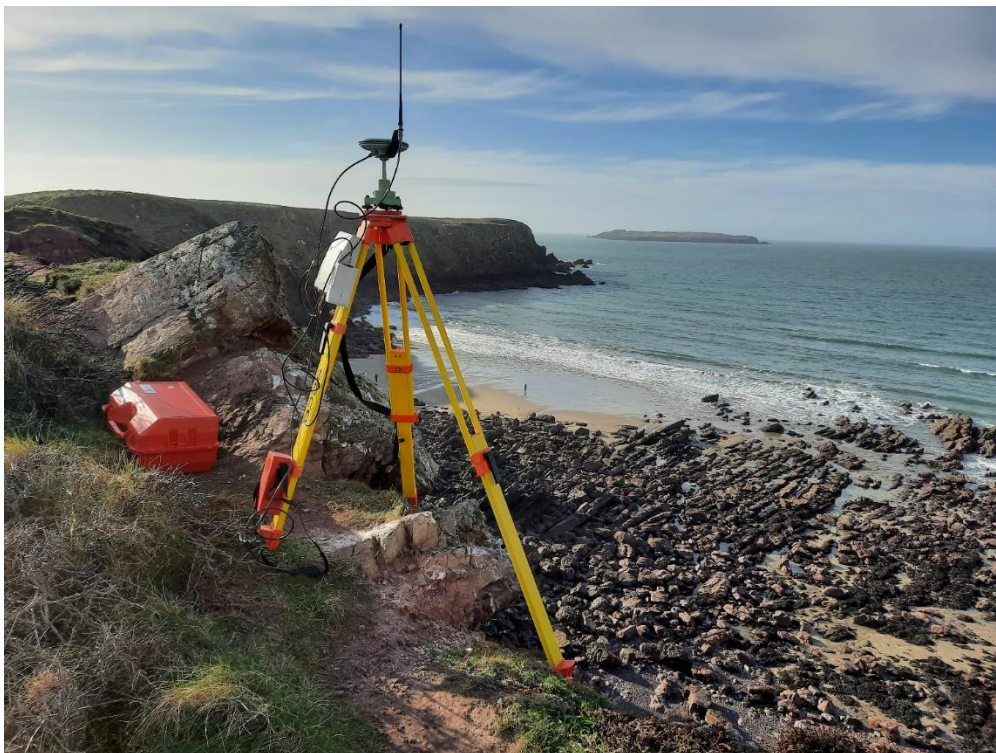
Example E2 GNSS tripod setup.
