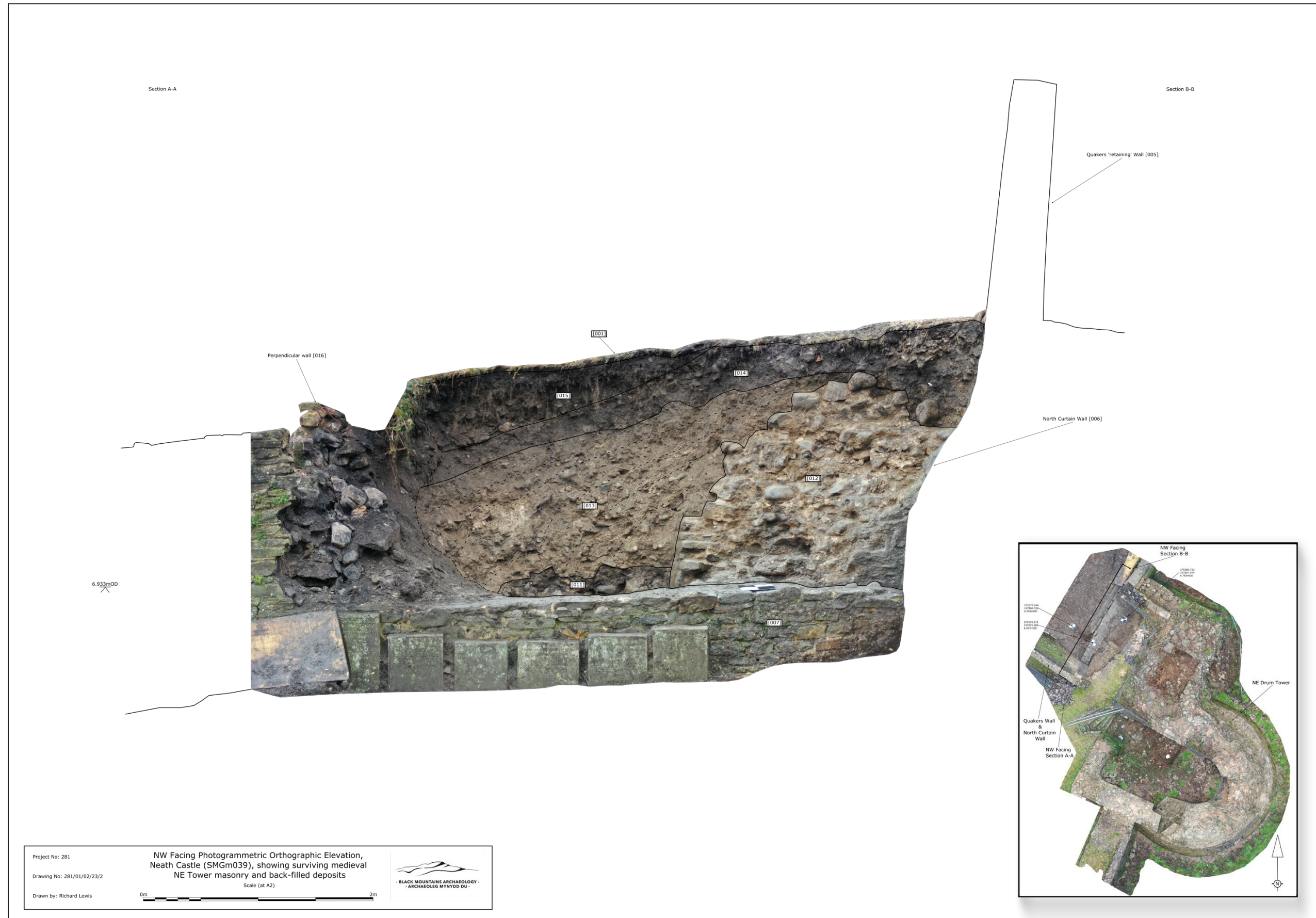
Figure 6. Post-excavation 3D photogrammetric orthographic elevation showing the masonry of the Northeast Tower [012], medieval deposits (011) and later back-filling deposits (013, 014 and 015), Neath Castle (SMGm039).
