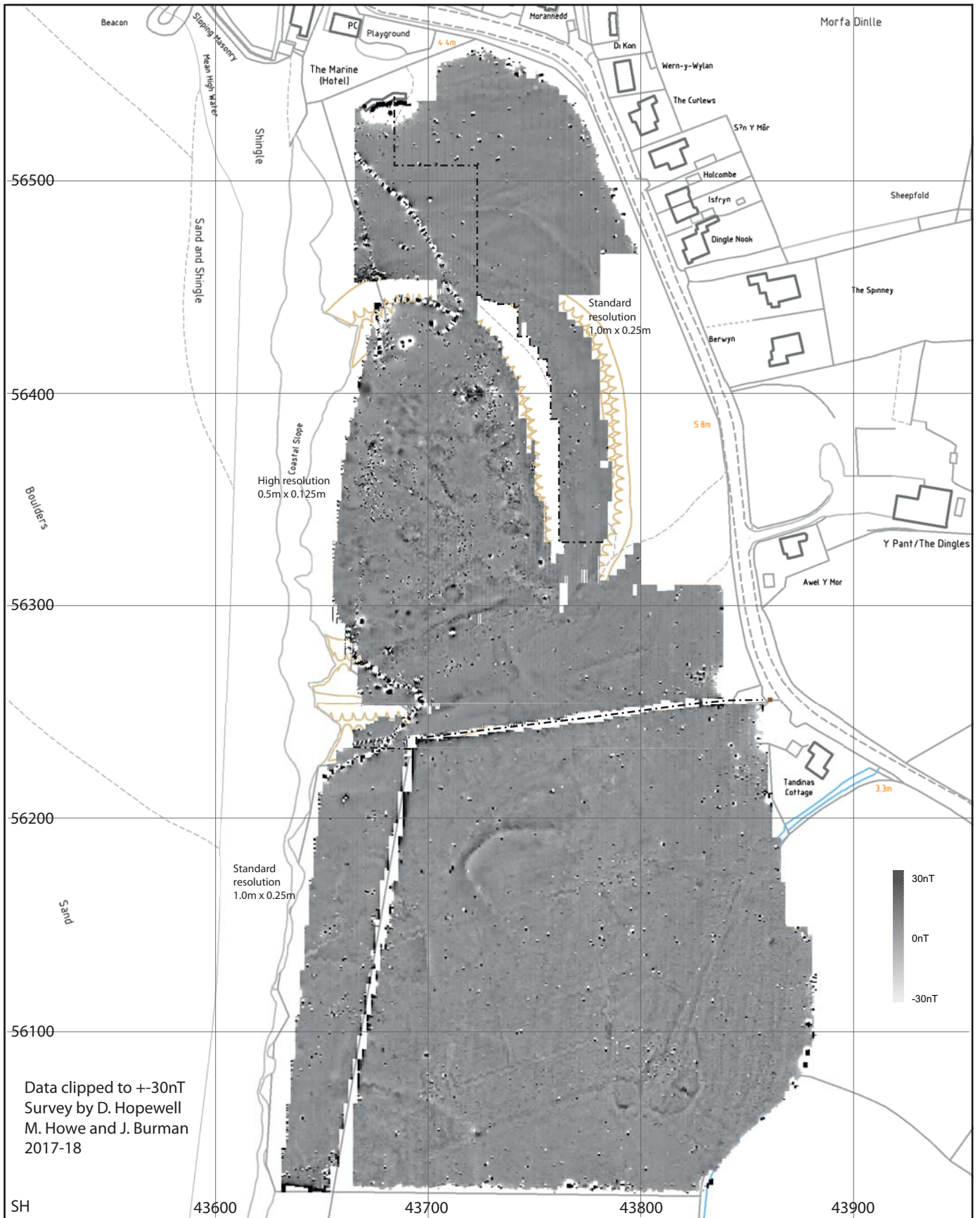
Fig. 8 Dinas Dinlle fluxgate gradiometer survey - grey-scale plot, raw data clipped to +-30nT
