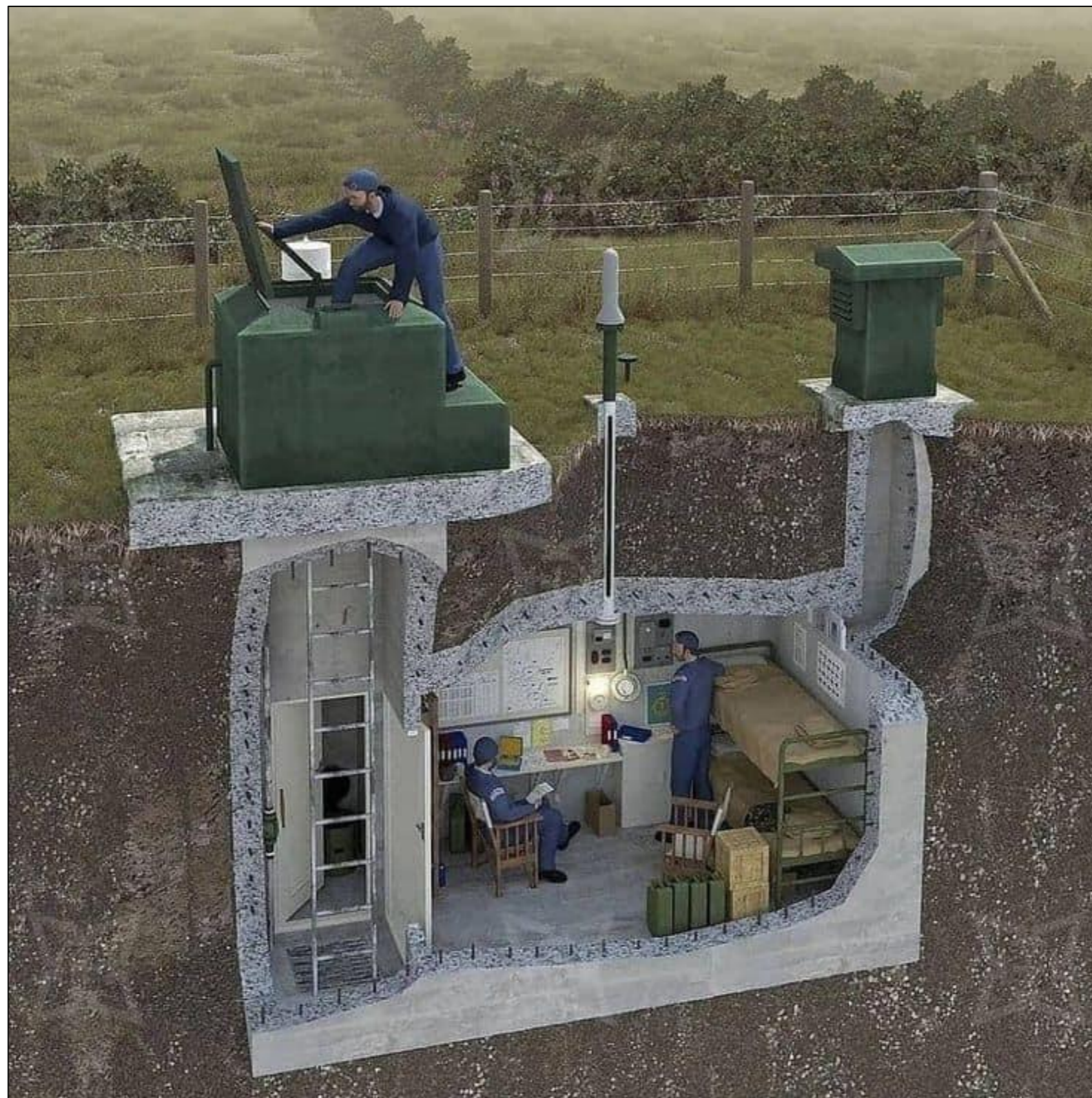
Plate 23. Three dimensional illustration of an ROC UGMP when in use (copyright Bob Marshall)
