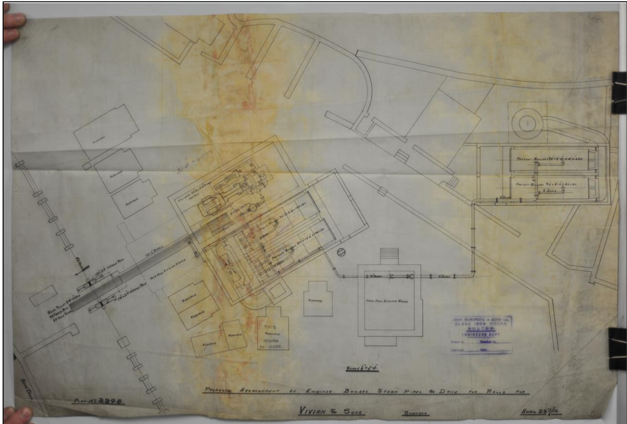
Plate 89. Proposal 2248 April 28th, 1910, showing position of original boiler range, near foot of remaining octagonal based chimney (copyright Swansea Museum)
