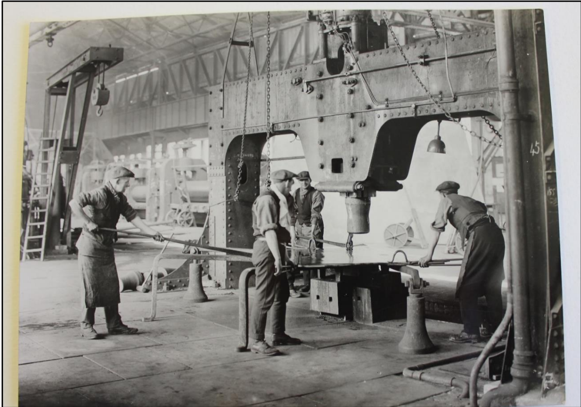
Plate 85. 20 th century photograph of interior of Hafod Plate Rolling Mill, possibly depicting the plate flattening machine in operation (copyright West Glamorgan Archives)
