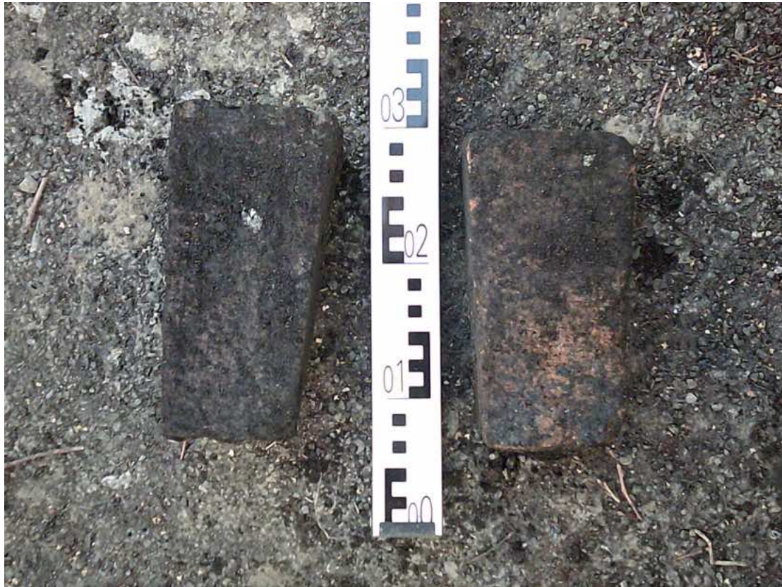
Plate 25. Examples of arch bricks recovered from weighbridge infill deposit (1402) in Test Pit 14.
