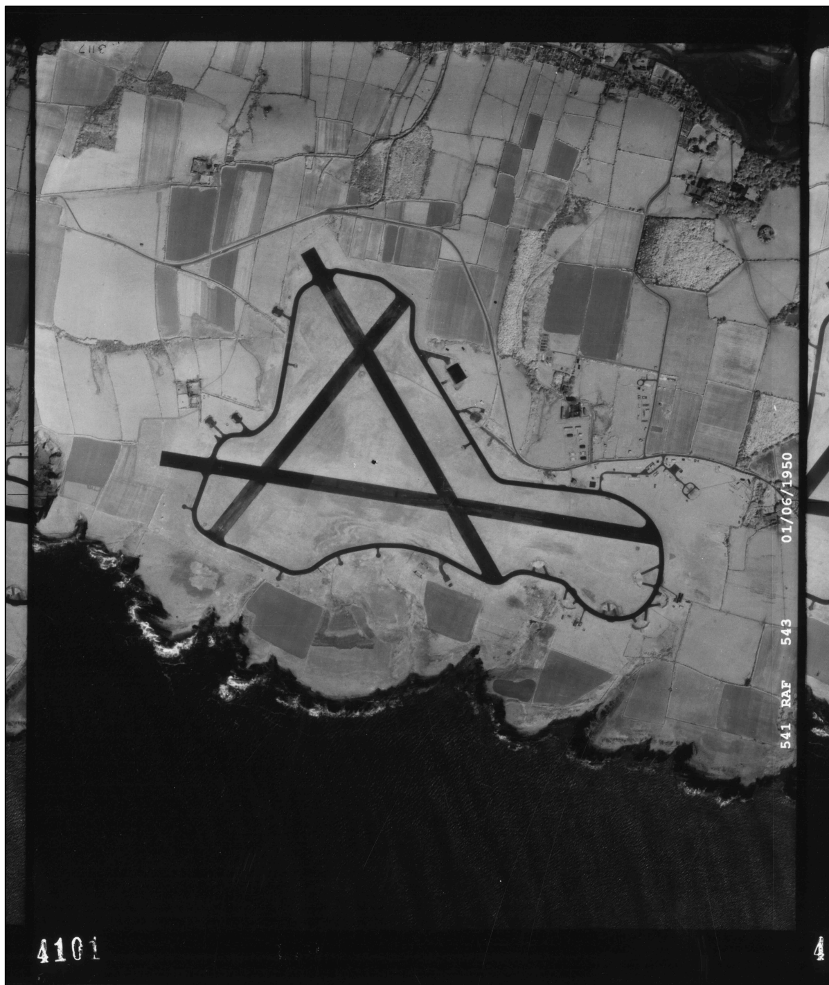
Plate 1. Aerial Photograph from 1950 showing Angle Airfield in a good condition. The six dispersal pens are visible in the south east corner. © Central Registry of Air Photography for Wales
