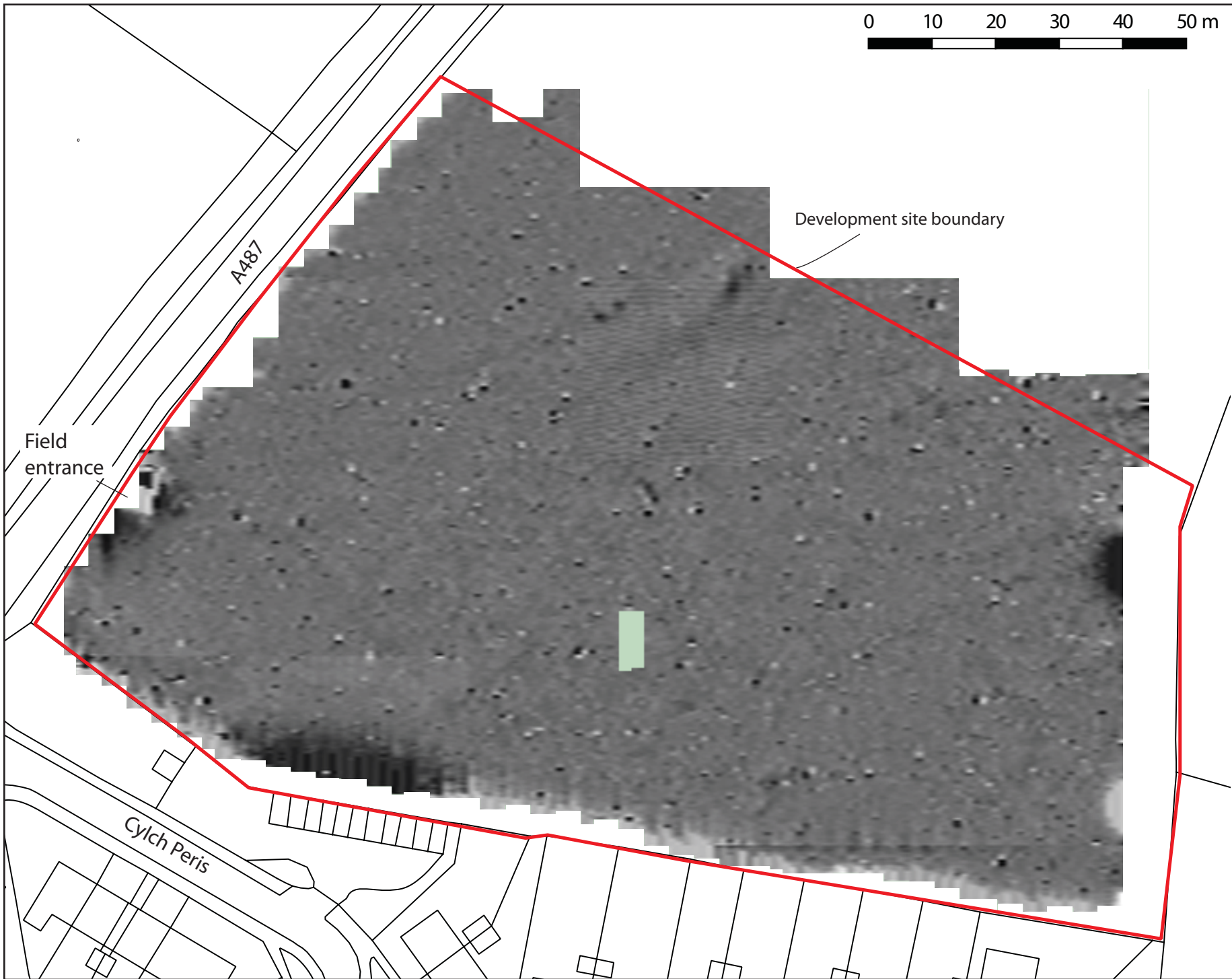
Figure 3: Processed geophysical survey results, overlaid with topographical detail. The survey has been destriped, and clipped to a range of +/- 10nT 1:800 @ A4.
