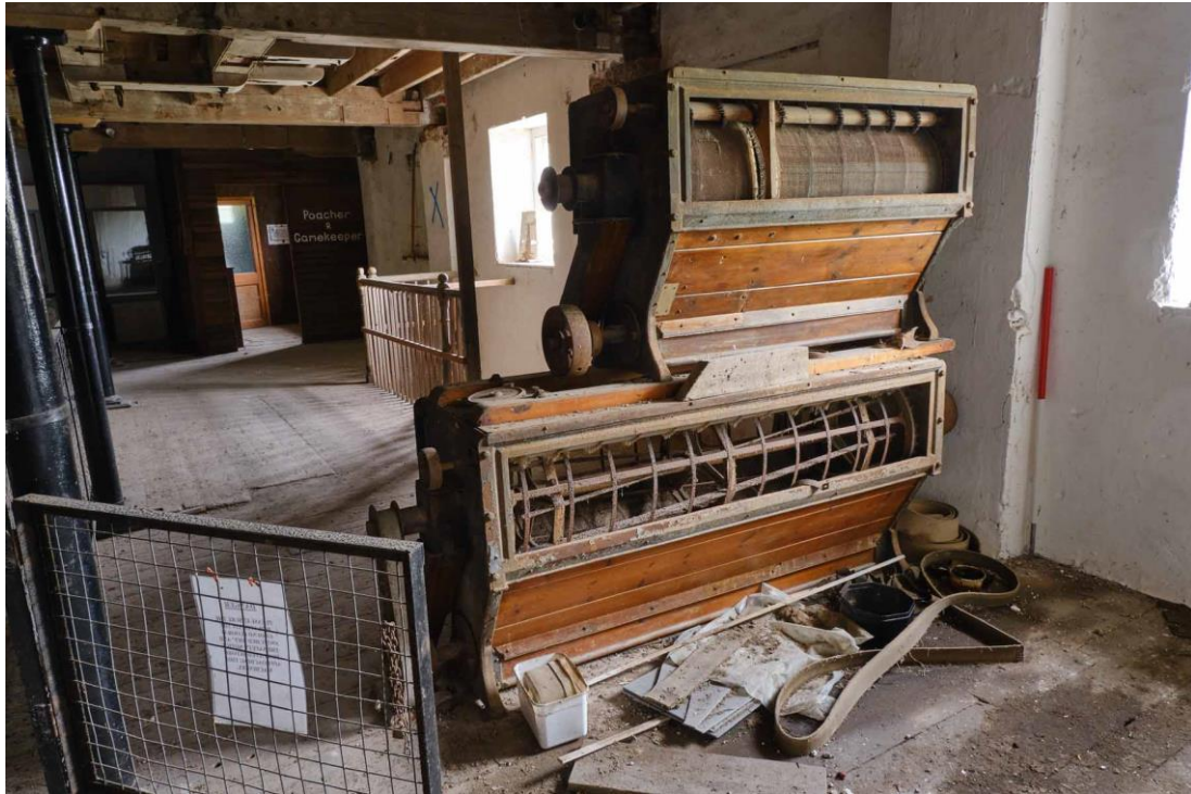
Figure 23. Armfield scalper on first floor.
