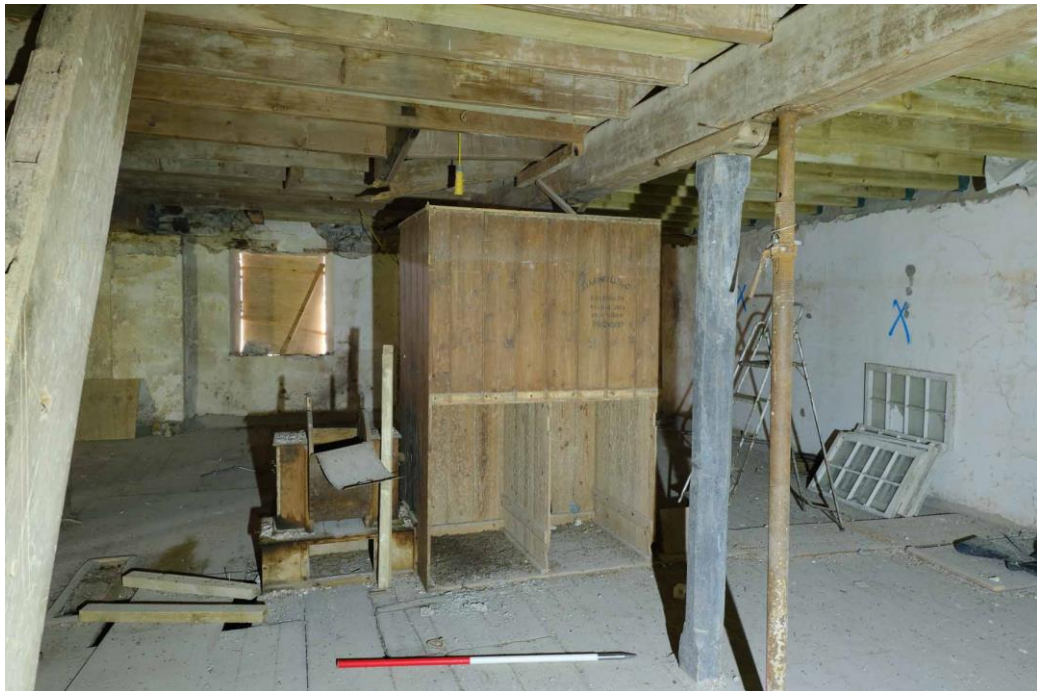
Figure 22. Grain separator, with fan on the left side, third floor.
