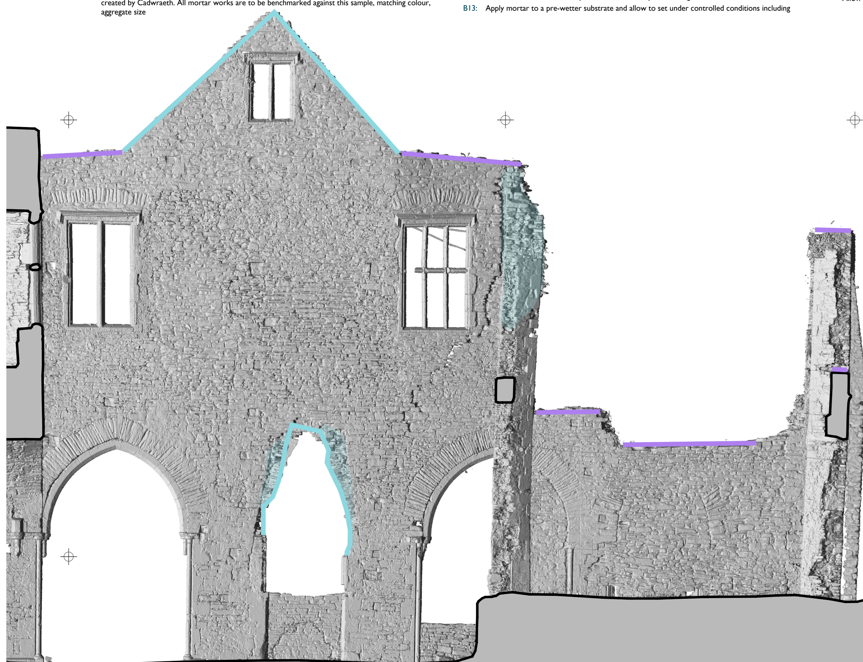
1 Elevation 1.2.4 and 1.2.8 (West face) 1:50 QUANTITY OF WORK - ELEVATION 1.2.4 and 1.2.8 A: Wall capping - stone slabs = As indicated B: Wall capping - mortar works = As indicated Da: Repointing to random coursed pennant stone = 90% Db: Repointing to dressed ashlar stone = 100% ; Dowel pinning = Allow 50dowels E: Removal of vegetation = As indicated
