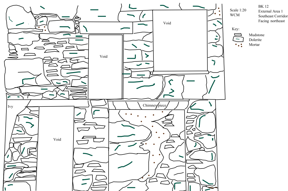
Figure 6: Elevation plan of External Area 1 of the Lower House showing two stories, window and doorways. Drawing: WCM and digitised by S. Doherty
