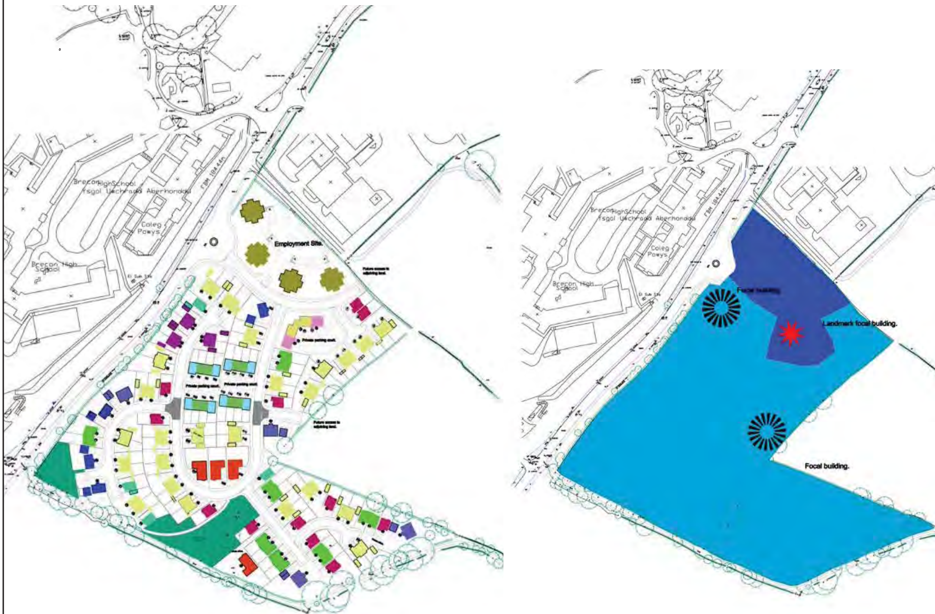
Figure 2: Outline proposed site development plans, showing a proposed layout of buildings and open spaces on the left, and building heights on the right.
