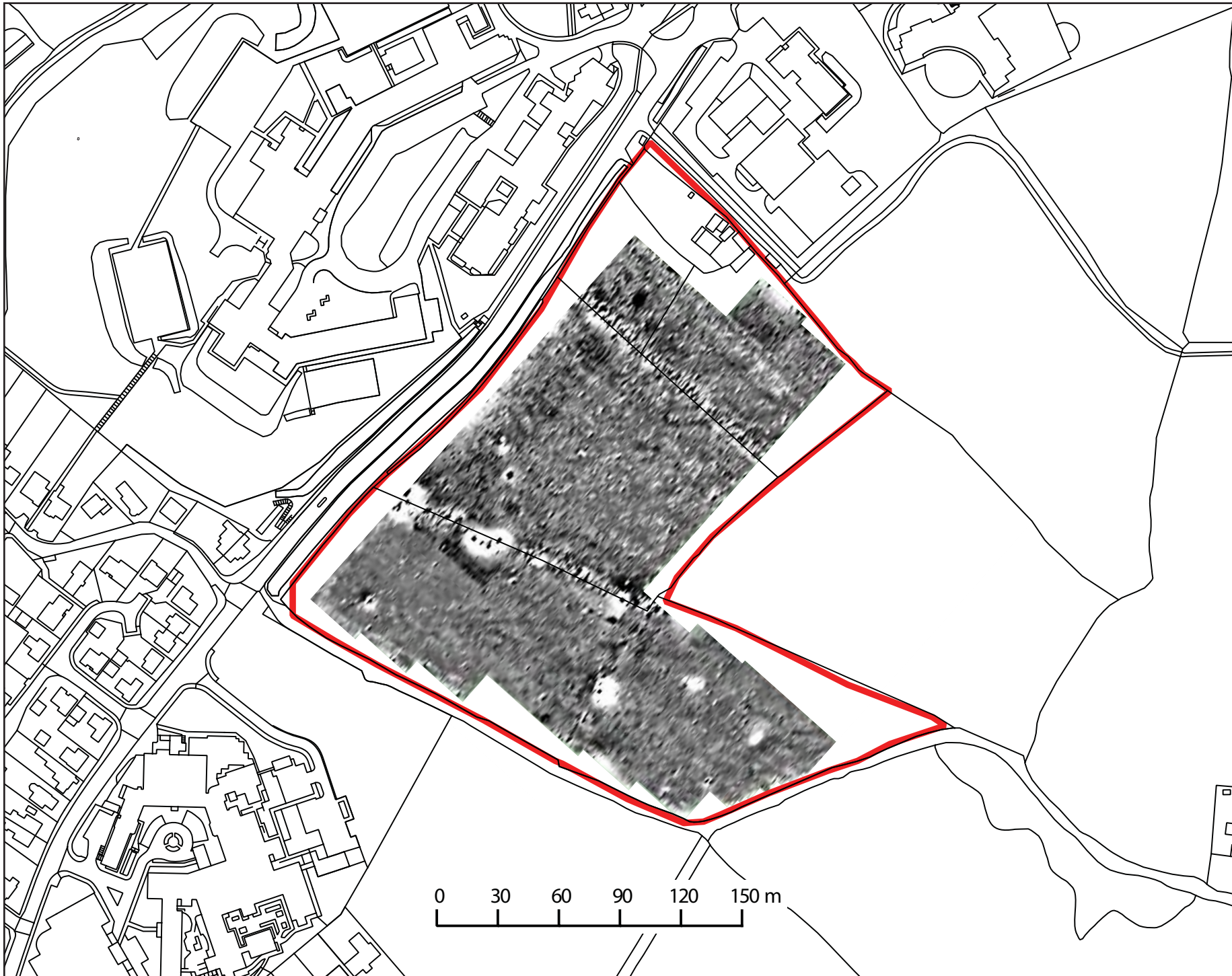
Figure 4: Geophysical survey results (clipped to +/- 3nT) located within the proposed development site (outlined in red).
