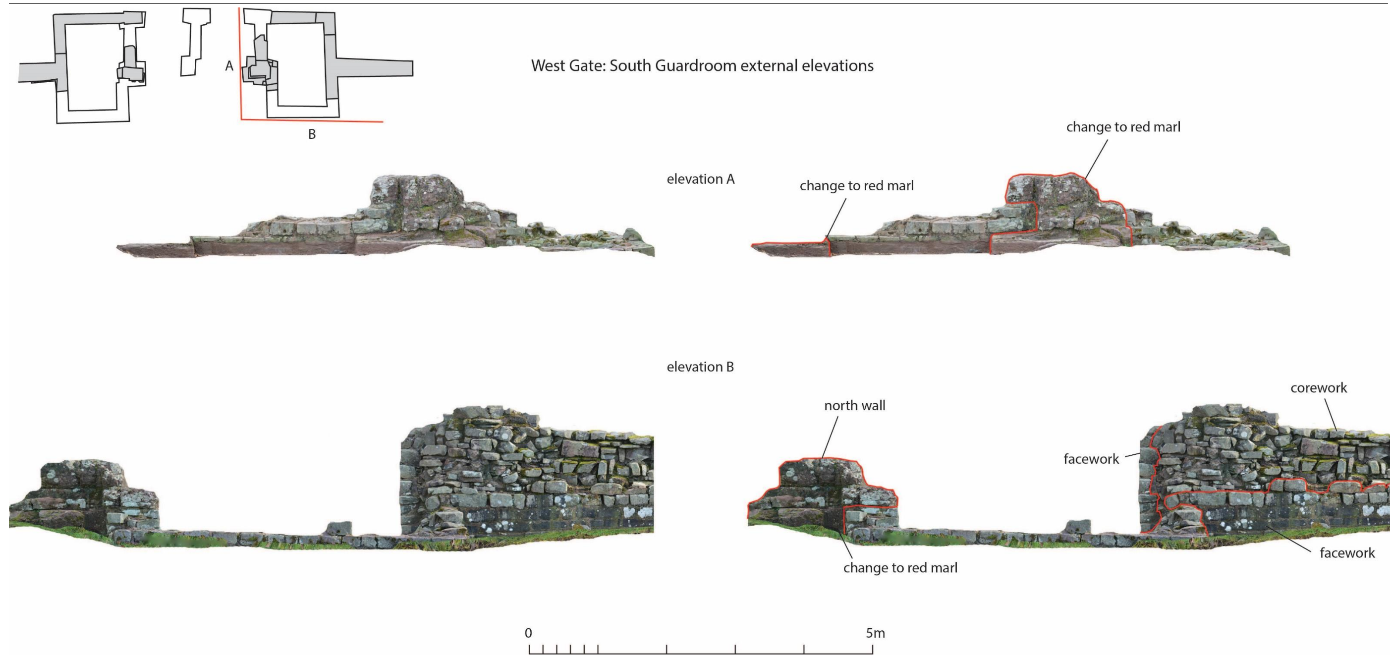
Fig. 13 West Gate: South Guardroom, external photogrammetric elevations
