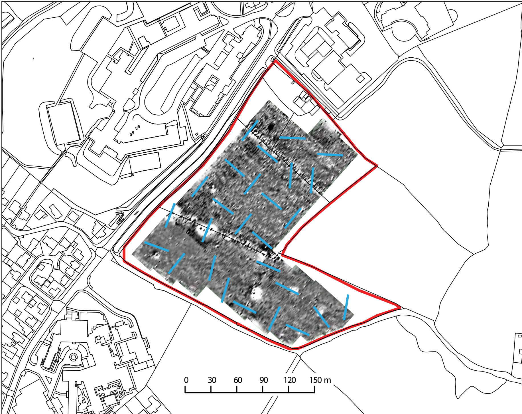
Figure 4: Trench location plan (Trenches in blue), overlaid on the geophysical survey results (clipped to +/- 3nT). Proposed development site outlined in red.
