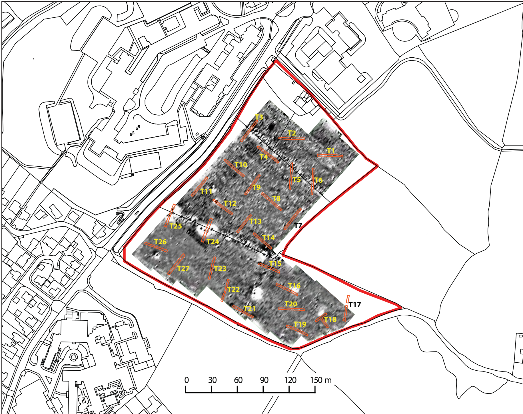
Figure 2: Site location (outlined in red) and trench location plan (Trenches in orange), overlaid on the geophysical survey results (clipped to +/- 3nT).
