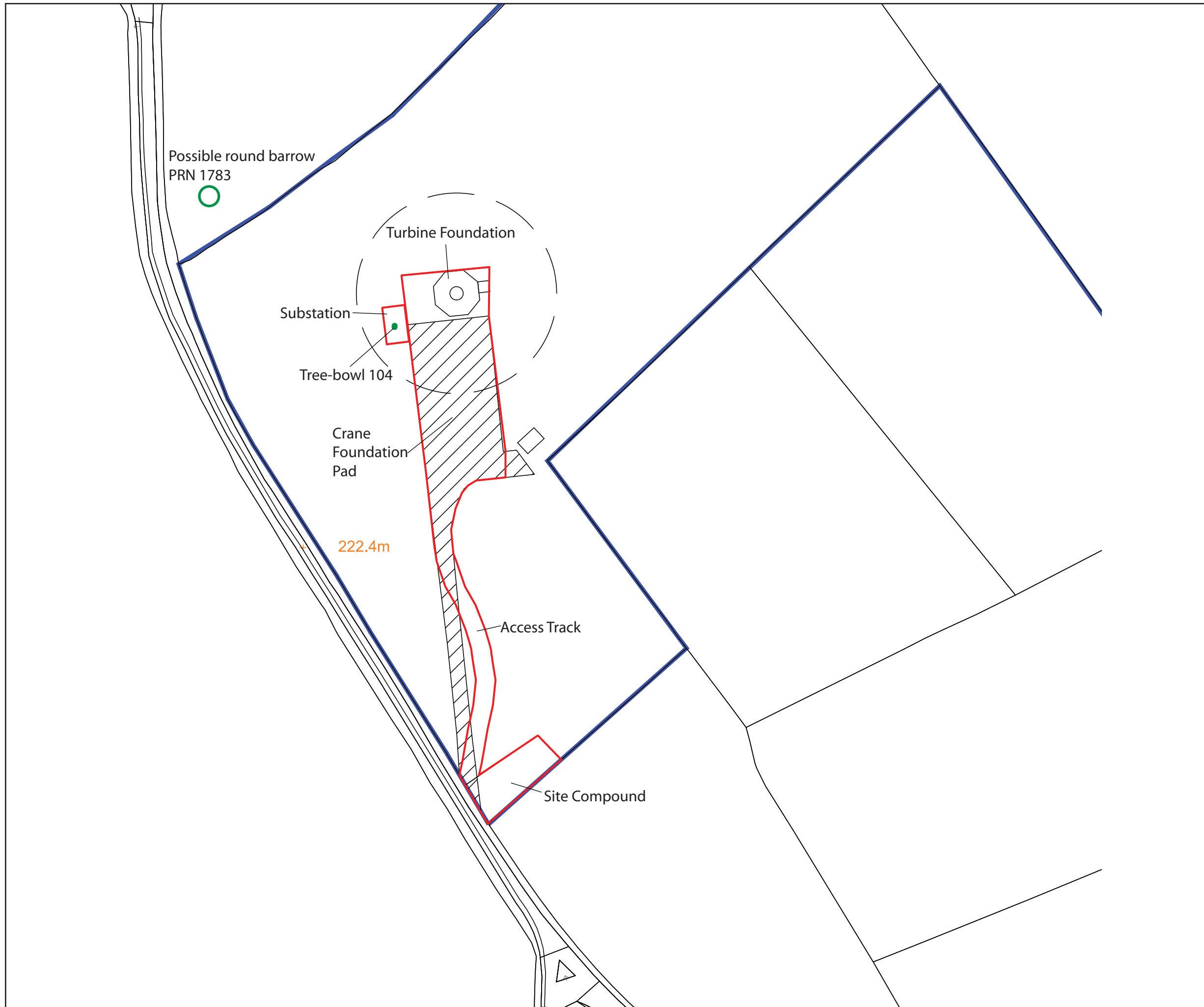
Figure 2: Development plan, showing the areas of groundworks as plotted during the archaeological watching brief in red, with areas labelled according to the description in the main text. This is overlaid on the original development plan as produced by Seren Energy (drawing number WWTSP02C).
