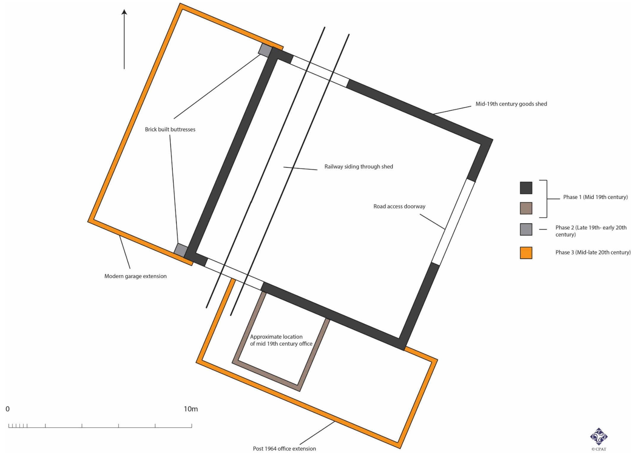
Fig. 10 Phased plan of the building complex
