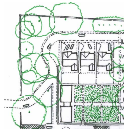
Illustrative scheme of 3-storey houses (circa 2,000sq.ft. dwellings) with 4 new flats (circa 750sq.ft. each), new secondary access and green space.
