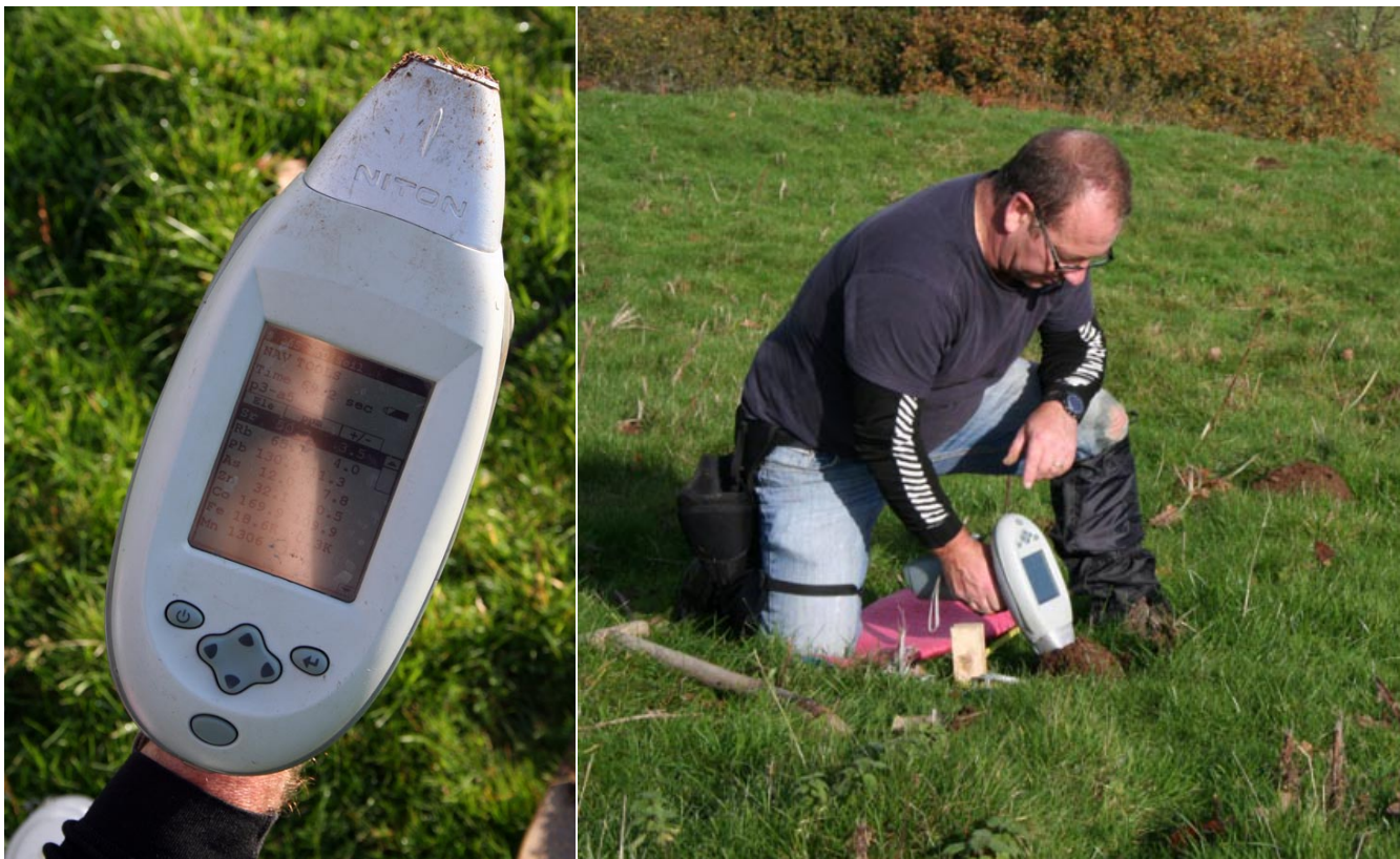
Figure 2. The handheld pXRF Niton XLt 700 analyser, at Castell Grogwyion (Crown Copyright RCAHMMW).
