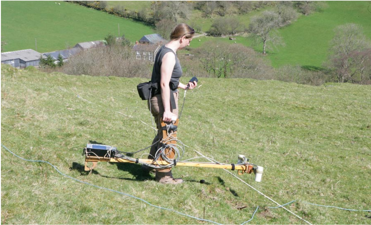
Figure 5. Anne Roseveare of Archaeophysica undertaking caesium magnetometry at Castell Grogwynion, March 2012 (Crown Copyright RCAHMW).
