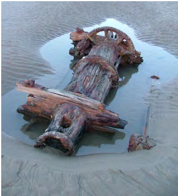
Figure 7: windlass possibly from the Brig MORINGEN (images courtesy Robin Ellis, Aberystwyth Civic Society and Nick Cooke, Wessex Archaeology)(NPRN 272432)
